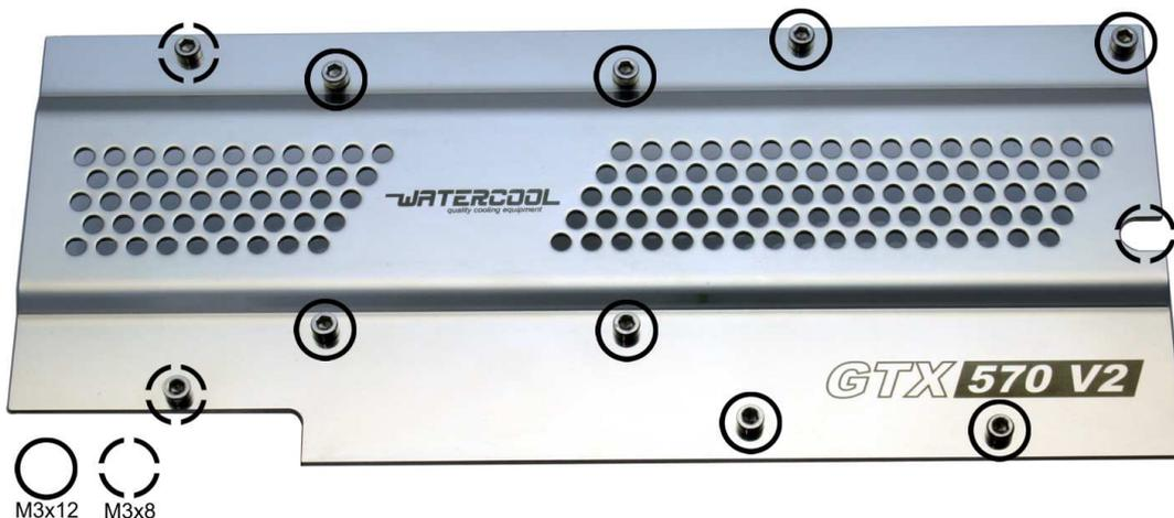
An Allen wrench size 2.5, M3x12 and M3x8 screws are required for assembly. The Allen wrench and the M3x8 screws are part of the delivery scope of the graphic card cooler; the M3x12 screws are included in the delivery scope of the back plate.
