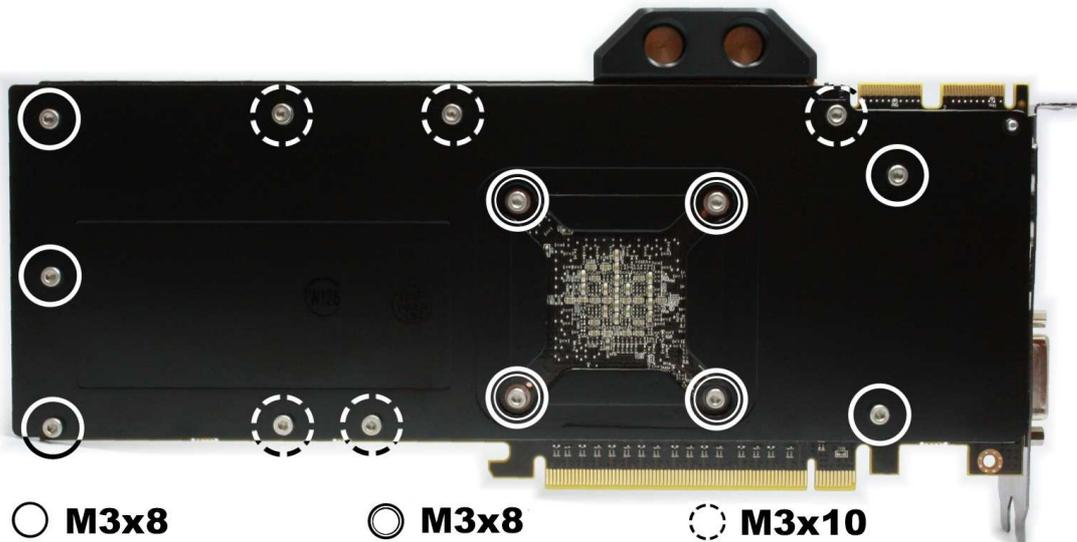
The cooler can also be operated without the original back plate. Should you prefer this type of assembly, only install the M3x8 screws and the washers.
